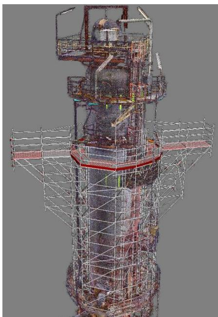
Bild 2: Using 3D scaffolding design, it was possible to precisely plan the unusual scaffolding construction at a height of 65 meters
