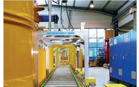
Roller conveyor with integrated decapping / capping station
