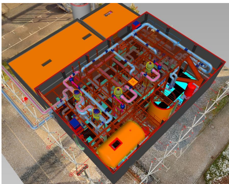
3D model of the new energy center including four heat exchangers that feed the waste heat as well as the heat from combined heat and power generation from Henkel into the district heating grid.
