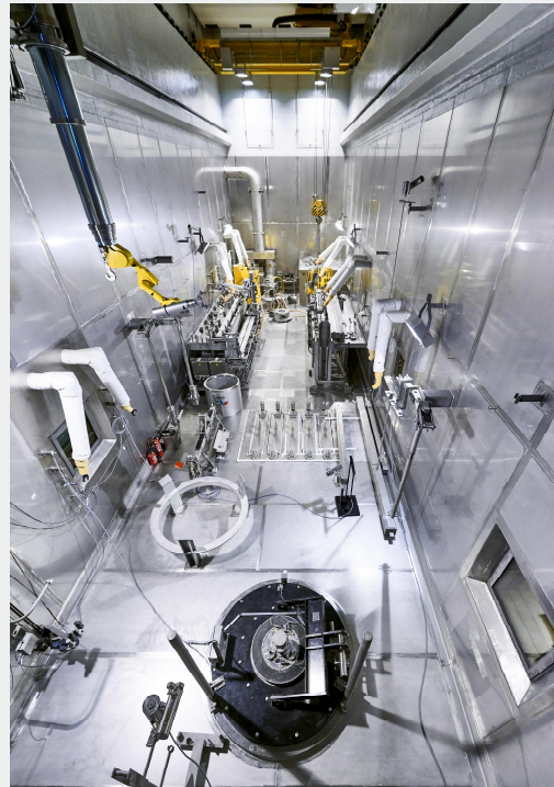
Typical application for remote controlled grab devices (hot cell of ICEDA Lyon-Bugey, France)
