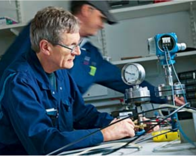
Technicians from Bilfinger Industrial Services regularly calibrate the pressure gauges for the plants. "It's all about protecting our people, the environment and our substances," says Regula Suter, Head of Production Support at Siegfried.
